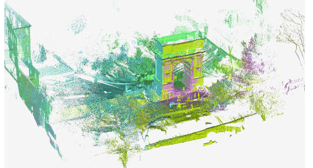
Figure 6: Urban data set with four scans positioned around a Roman arch. Notice the artefacts caused by moving people in front of the arch. For better visibility, only 25% of the points are displayed.
