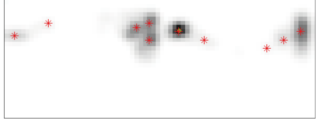
Figure 2: Example of a smoothed 2D histogram of all possible solutions with the ten detected local maxima (red) and the true solution from the ground truth (green). Abscissa: 3D rotation angle; ordinate: 3D translation.
